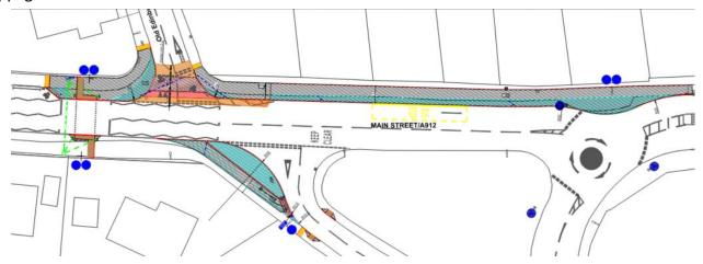
The changes to traffic movements and vehicle priorities vs cyclists and path users are the key aspects of the project. By altering the infrastructure in this area all users of the space are required to slow down and take due notice of the priorities. The new layout has begun to work as drivers read the road correctly, become familiar with the changes and use the area as designed.
